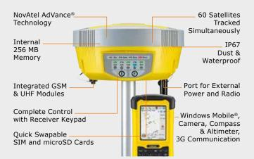
Zenith10/20 receivers are future proofed, benefitting from world class NovAtel AdVance® technology that supports GPS, Glonass, Galileo and BeiDou GNSS systems.
